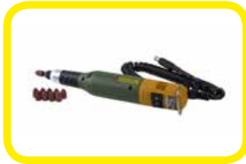
Grinding equipment to remove paint on the radiator
