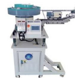
Housing inserting station
