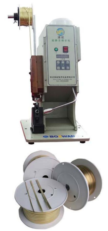
Matching with brass belt machine, it is used for the connection among nude wires, with good conduction and wide application.
