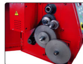
127T gear enable both metric and imperial thread cutting
