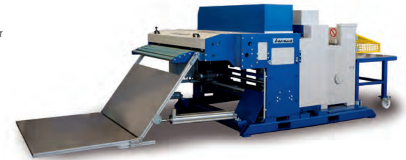
Image shows feed table liftable and run-out table
