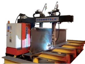
WA 1000 / WA 1500 • Automatic fillet and butt welding with joint tracking • Multipass welding
