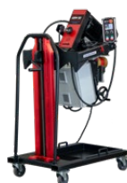
ABM-50 • Bevel width up to 50 mm • Top and bottom beveling • Auto feed mode • Bevel angles: 15-60°
