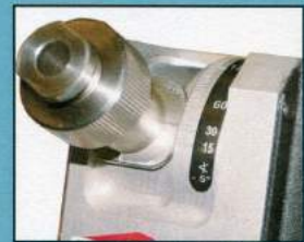
Eccentric plate triples the use of the diamond wheel.
