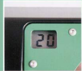
The grinding angle is shown in the digital readout.
