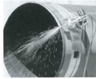
Pipe flame cutting machines for pipe \text{\O} 10'' to 120''
