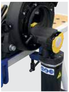
Second saw blade position to cut off elbows
