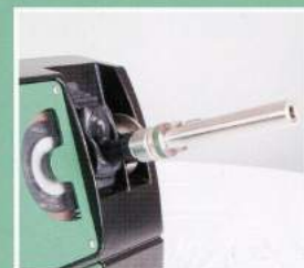
The tip is easily flattened, by setting the grinding angle at 90°.
