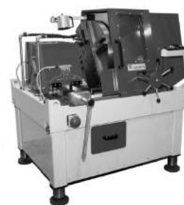
PBM Pipe end preparation machines for pipe \text{\O} 2'' \text{ to } 30''
