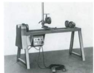
Welding manipulation and roller standards - electric driven
