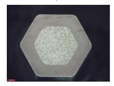
Terminal cross section diagram
